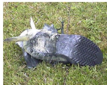
BfR Combat Boot after 70g explosion on heel
