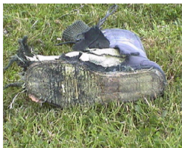
BfR Combat Boot after 50g explosion on ball
